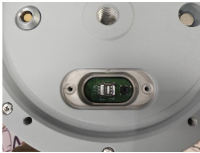
Figure 6. A300L SIM Card Cover: Removal and Installation
